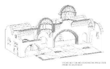
Fig. 8: Trapeza church, axonometric projection from the southwest showing 14th century dome (left) and 16th century dome (right) (projection by Joanna Ostrowska)
